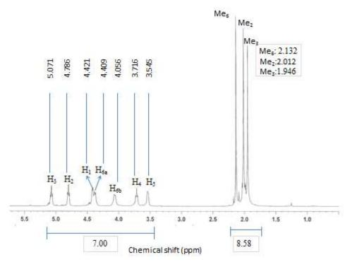
**Fig. 3.** <sup>1</sup>H-NMR spectrum of cellulose triacetate (DS = 2.86) produced from cotton fibers (CF). Me refers to methyl protons in acetyl group, H to protons on anhydroglucose, and subscripts to positions of Me or H on the anhydroglucose.
