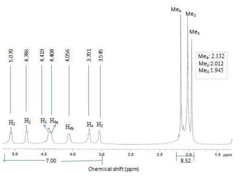
**Fig. 4.** <sup>1</sup>H-NMR spectrum of cellulose triacetate (DS = 2.84) produced from recycled writing papers (RWP). Me refers to methyl protons in acetyl group, H to protons on anhydroglucose, and subscripts to positions of Me or H on the anhydroglucose.
