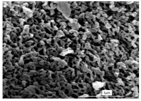
Fig. 10. SEM micrographs of cellulose triacetate produced from recycled writing papers
