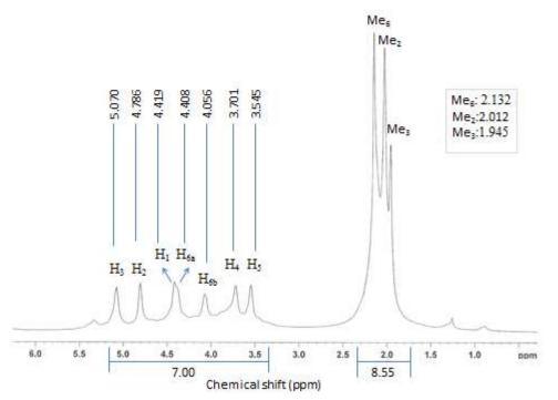
**Fig. 5.** <sup>1</sup>H-NMR spectrum of cellulose triacetate (DS = 2.85) produced from recycled newspapers (NP). Me refers to methyl protons in acetyl group, H to protons on anhydroglucose, and subscripts to positions of Me or H on the anhydroglucose.
