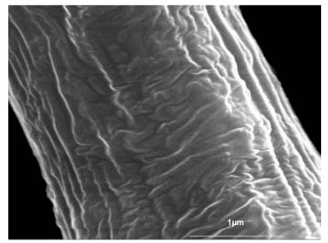
Fig. 8. Cotton fiber (CF) upon acetylation to form cellulose triacetate (CTA) (89,705X)
