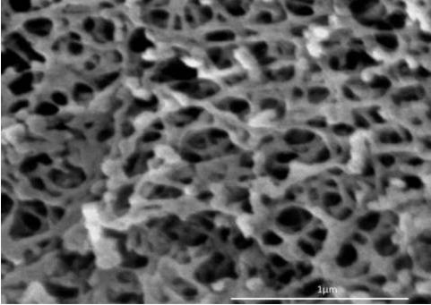
Fig. 9. SEM micrographs of cellulose triacetate produced from cotton fibers
