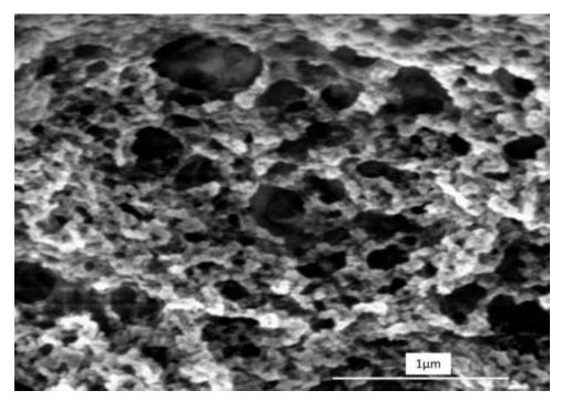
Fig. 11. SEM micrographs of cellulose triacetate produced from recycled newspapers
