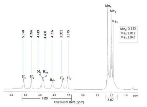
**Fig. 6.** <sup>1</sup>H-NMR spectrum of cellulose triacetate (DS = 2.89) produced from macerated woody fibers (MWFL) of *Leucaena leucocephala.* Me refers to methyl protons in acetyl group, H to protons on anhydroglucose, and subscripts to positions of Me or H on the anhydroglucose.
